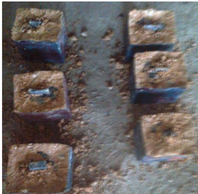
Appendix B: Image showing the Crucible Containing the Case-hardening Mixture after offloading from the Furnace
