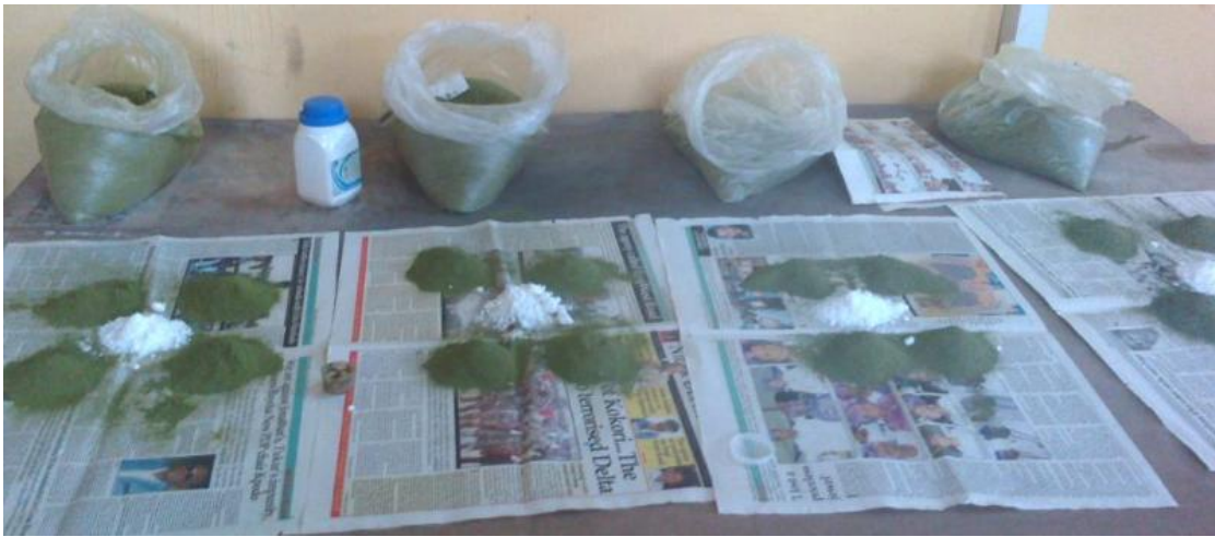
Appendix A: Four Volumes of Cassava Powder (green heaps) and One Volume of Barium Carbonate Energizer (white heaps)
