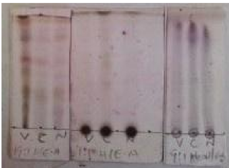
Fig. 1. TLC plates; left=hexane, middle; ethyl acetate, right; methanol extracts
