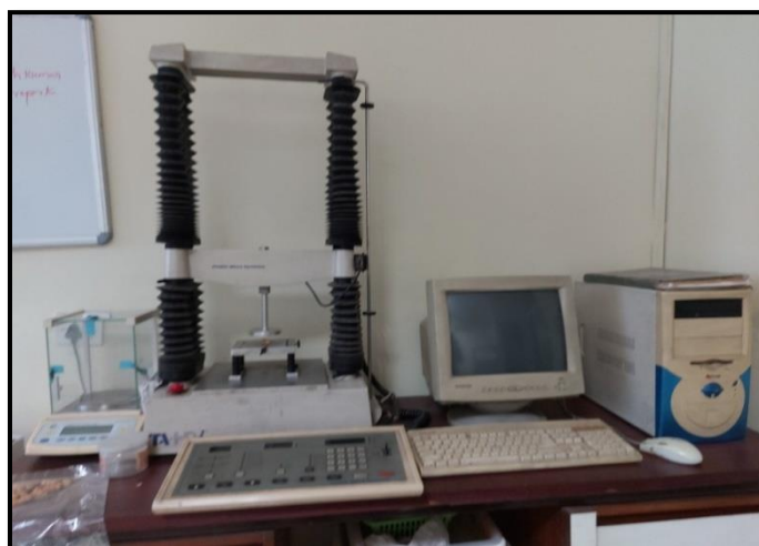
Fig. 5. Determination of rupture force of groundnut pod on Texture analyzer
