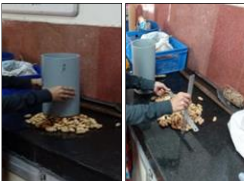
Fig. 4. Determination of angle of repose of groundnut pods
