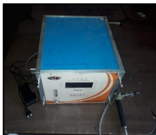
Pic. 1. Gas board analyser
