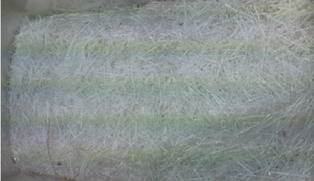
Fig. 1. Barchip fiber used in the study.
