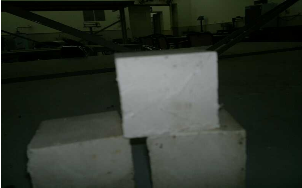
Fig. 2. Cubes 50 mm used for compressive strength tests.
