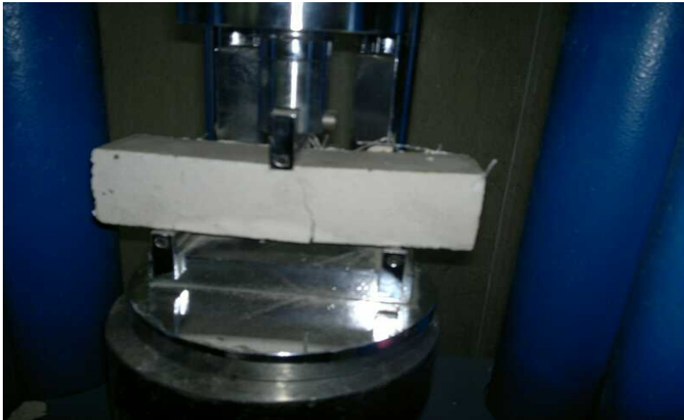
Fig. 3. Prisms 40 ×40×160 mm used for flexural strength test.
