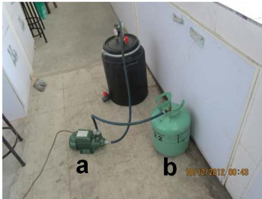
Fig. 1. Showing biodigester and a) Surface pump, (b) Gas cylinder
