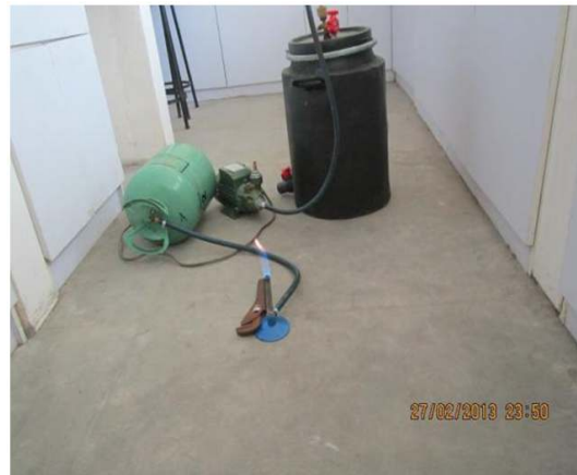
Fig. 2. Generated biogas used to light a Bunsen burner
