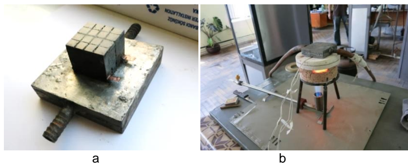
Fig. 7. a - thermoelectric module connected to water cooler, b - thermoelectric module testing.
