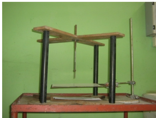
Fig. 6. Electrode Stand T_G with the barrier carrier
