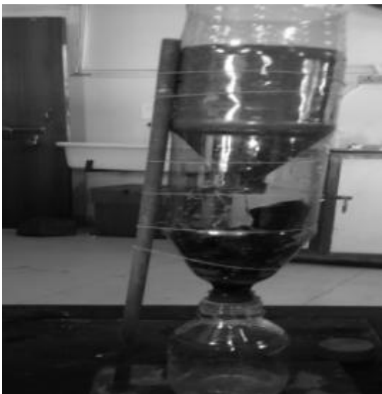
Fig. 2. Sand bead and coal bed apparatus
