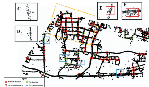
(b) Results of road intersection detection in data 2
