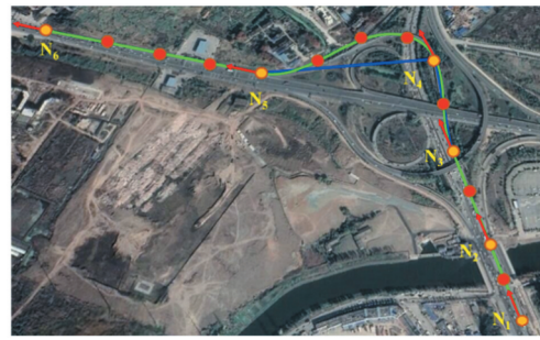
(b) Clothoid-based resample result of a trajectory
