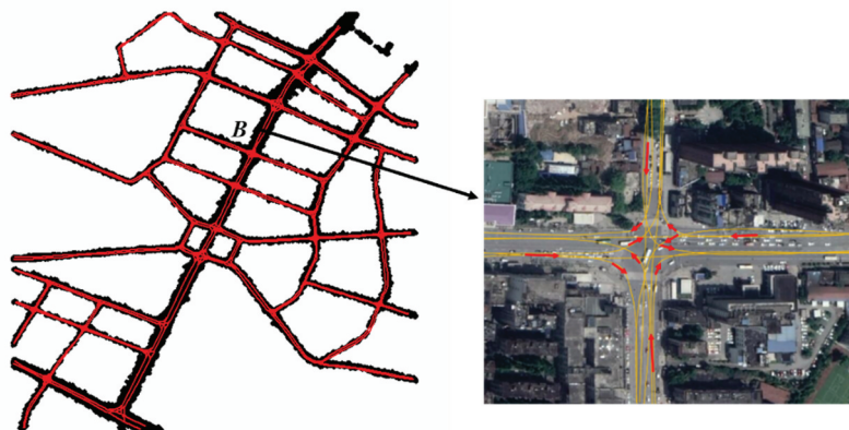
Figure 17. Centerline extraction results of data 1.
