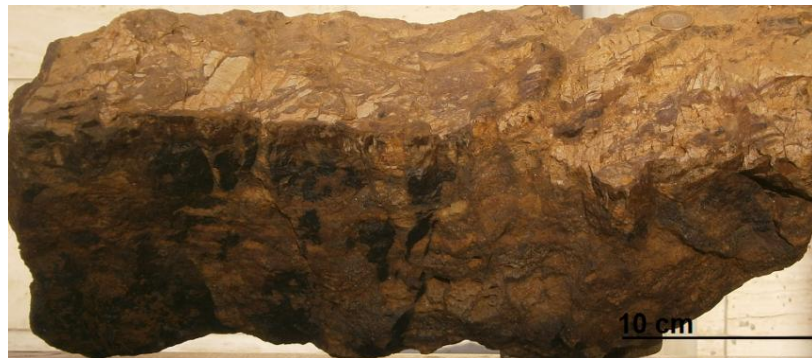
Fig. 6. Magnetite-apatite ore: Magnetite (dark) and apatit crystals (light) of different growth and directions with some chlorite on the bottom
