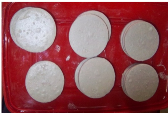
Fig. 2.1. Some of the fired samples formed by wet and dry pressing forming methods
