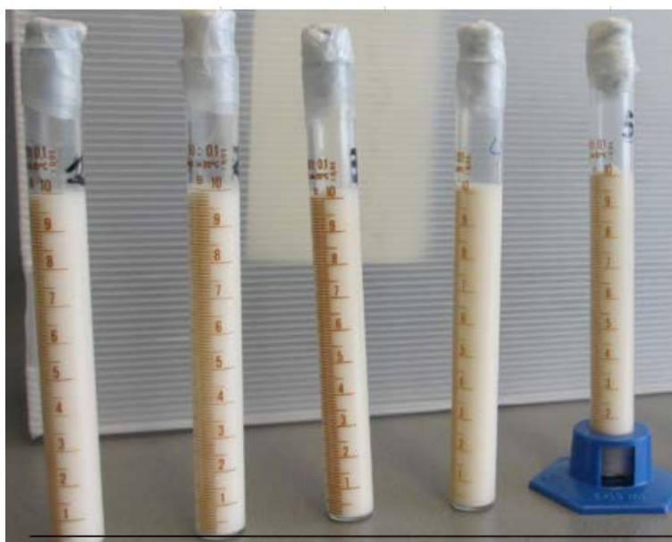
1 ml = 50/8 mm height. Initial height in gravity drainage of 10 ml (62.5 mm).
