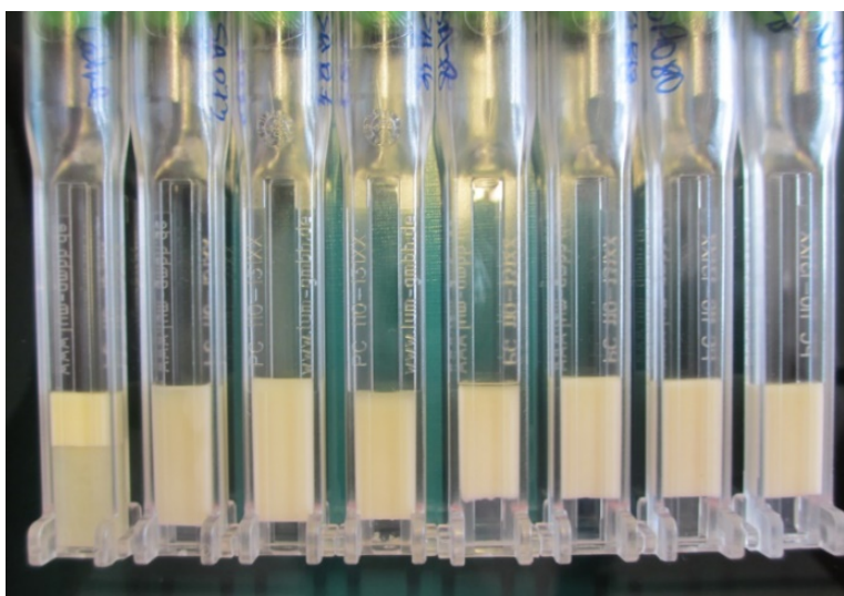
Figure 10. Samples that have run for 24 h at 4000 rpm. These samples showed the impact of varying structurants in some typical pourable dressings.
